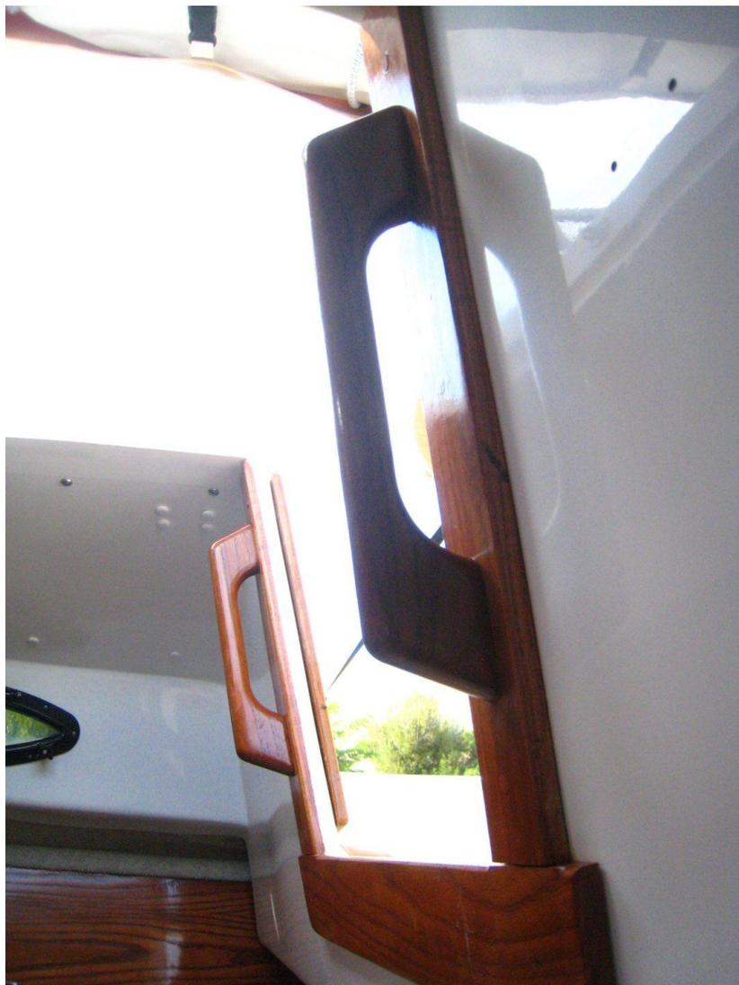
Then it was spring time and the original plywood hatchboards are looking lame. I bought a two foot piece of teak and sliced into three boards and made new solid teak hatch boards that look much better and have a far richer grain pattern.
