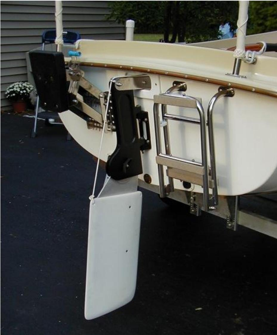
My situation with the new rudder is as follows. Mine came with the pivot hole drilled. Installation was just removing the pivot bolt and inserting the new rudder blade. However, the new rudder would not come fully down, like the original. I removed the new rudder and compared the shape of the rudder head on the new and the original. They were a little
