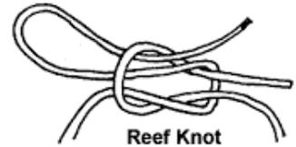
1. **Inhaul** - Tie the reefing grommet in the luff down to the tack grommet or gooseneck fitting with a short piece of line using a reef knot.
