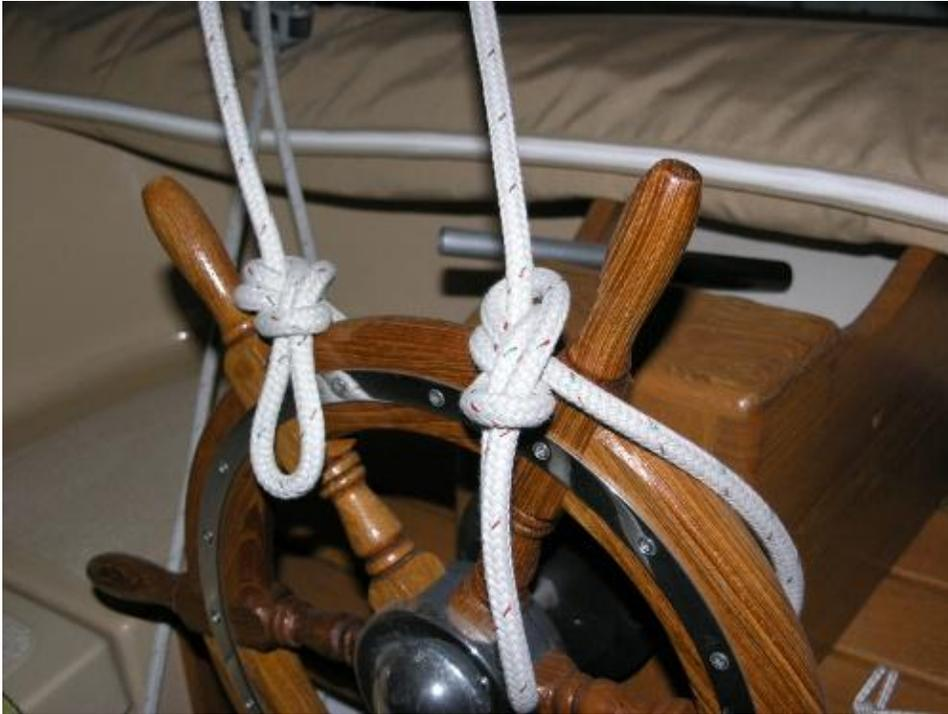
And here they are pulled up short into the block. If the boom were held up off the gallows by the lazy jacks I don't think it would swing back and forth at all, and the sheet wouldn't have to be drawn tight. The extra slack you see is in the parts of the sheet no longer able to take any tension because of the stopper knots:
