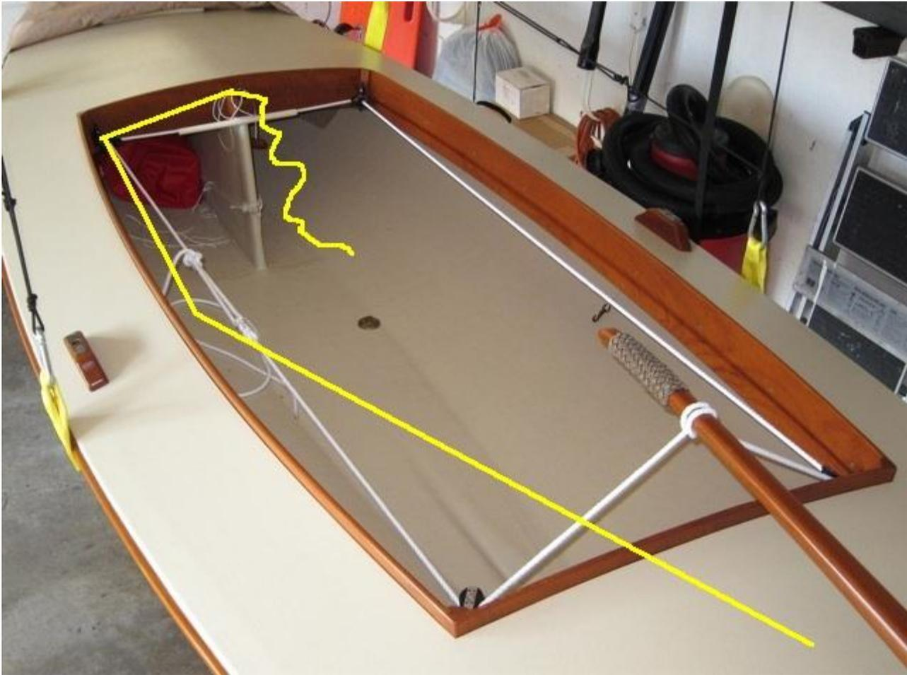
Here's a blow up of that area. The centerboard pennant comes up out of the block immediately behind its cleat and leads forward. There's room between the coaming and the c/b pennant hole to mount the little tiller cleat cross ways, leading left to right. It will be 90° to the pennant cleat.
