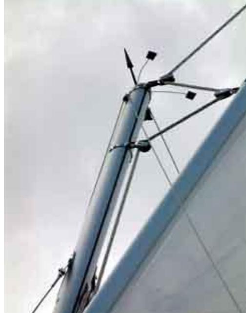
The eyestraps allow the line to move to either side of the sail. As a side note, we also use the lazyjacks when reefed to gather the sail up, instead of reefing lines. The black line on the boom is the single line reefing.
