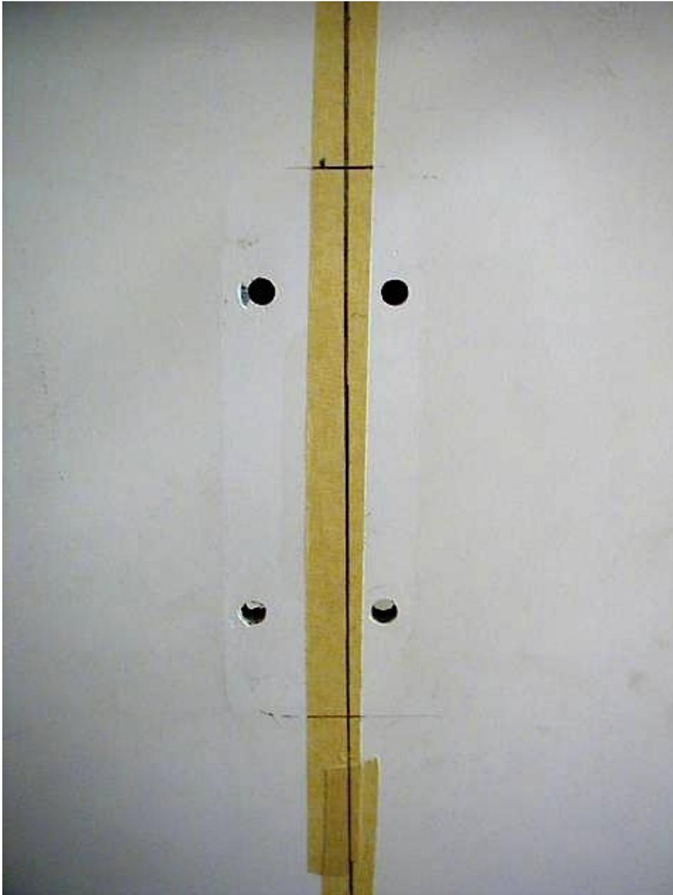
The rudder was mounted 5/16" to port and rotated 3° clockwise. I guess they were lucky just to get the it on the transom the day it was built. S o o o, haul out the glass filled epoxy, fill holes, drill new ones, and this time, mount the rudder with 1/4" aluminum backing plates, not just the thin washers it came with.
