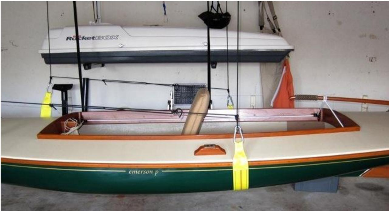
The Opti Air bags will have to move back under the side coamings so I will have leg room under the fore deck. The centerboard adjustment is easy to reach. The sheet will be led forward to the top pulley of the double block in the forward port corner, a short lead to my hand. There's room for a small clam cleat for the sheet to be mounted on the teak top of the centerboard trunk if I want to. The same one I removed from the tiller.
