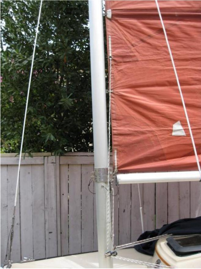
Here's how it look from the cockpit. I never have to leave the cockpit to reef and can reef down in about three minutes. I start the motor, head into the wind, maintain enough way to maintain direction, scandalize the gaff, lower the main halyard as I pull on the jiffy reef, set the two forward cleats, and then set the aft jiffy reef. Depending on conditions, and how I feel, I may tie the two center sail ties.
