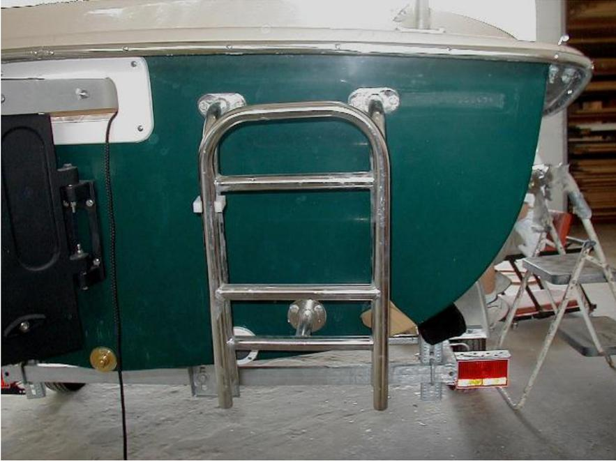
Here's the retracting motor mount. You can see it's mounted with only four bolts. The lower pair are in the uppermost of the three lower positions. I think the factory uses the same hole pattern for both the fixed and retractable motor mounts. You could email Gerry Hutchins at Compac to confirm that. I decided to fill the lower pair of factory holes, and drill new lower holes in the bottom position of the bracket, giving me the greatest spread possible.
