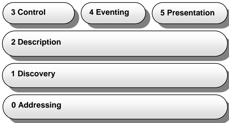
Figure 4: UPNP’s six layers of device functions: IP addressing, discovery, description of URLs and services, and optional control of other UPNP devices, event messaging, and presentation or the Web page for the device. Layers 0 through 2 exist in all UPNP-enabled devices.
